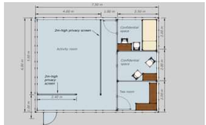
Figure SEQ Figure \* ARABIC 1 Suggested indoor lay-out. UNFPA, IRC (2017) Safe Spaces for Women and Girls Standardisation and Technical Guidance
