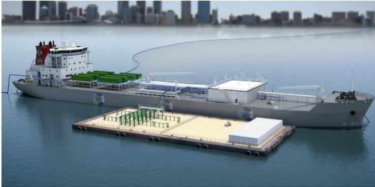
**The “Emergency Relief Vessel”** - Producing clean drinking water for the population in catastrophic areas, by converting seawater into drinking water. After earthquakes, tsunamis, flooding e.g. onshore-based water supply and water infrastructure is not able to provide the local community with sufficient drinking water.
