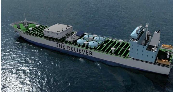
**The “Reliever”**- a converted ship that can treat wastewater, for example while a land-based plant is being modified, expanded or repaired. Typical need: a slightly developed country with unsatisfactory treatment capacity.
