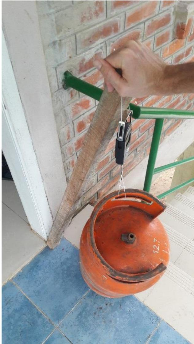
*How to weight the cylinder: with a 1-m pole, a weighting scale and a bit of rope. Wedge the pole in the against a solid support (e.g. a wall) and push gently it to weight the cylinder until the cylinder do not touch the ground anymore.*
