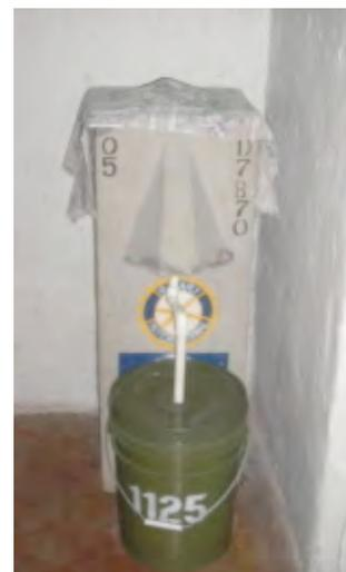
Figure 8: A concrete BSF (Pure Water for the World)
