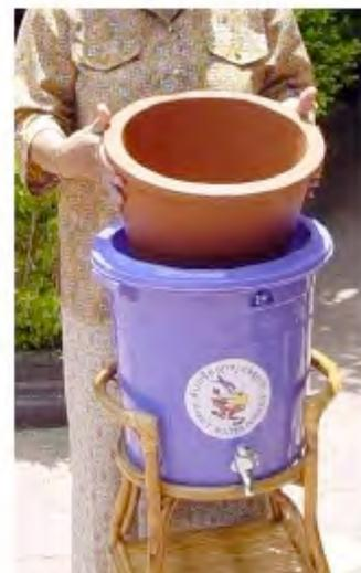
Figure 7: A ceramic filter (PFP)
