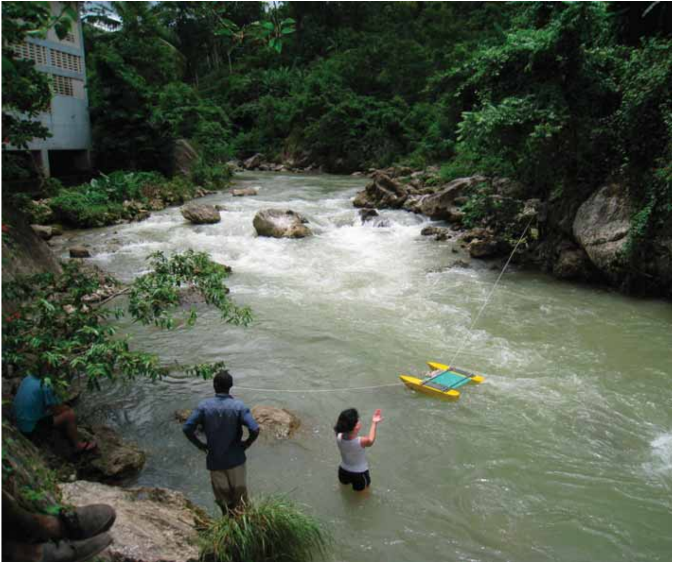
UNEP partners from Columbia University measure river flow velocity in support of a proposed run-of-river hydropower scheme in southern Haiti
